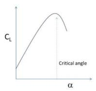
But once you increase a beyond the critical angle, which in a typical light GA aeroplane is about 16°, you'll get less lift no matter what else you do. So while increasing a up to the critical angle can give you Option 1, 2 or 3 above, once you increase a past the critical angle, all you'll get is Option 3. The airflow has separated from the wing. There's still lift, which is why you don't fall out of the sky, but not enough lift to stay level.
